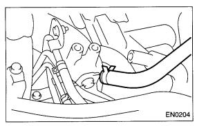
10) Connect the engine coolant hoses to the throttle body.
