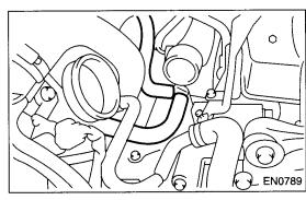
12) Connect the pressure hose to the intake duct.
