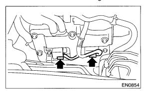
7) Connect the engine harness with clip (A) to the bracket.
