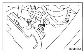
6) Connect the connector to the ignition coil.
