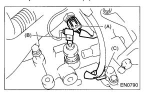
4) Connect the connector to the knock sensor.
