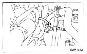
19) Disconnect the connector from the camshaft position sensor.
