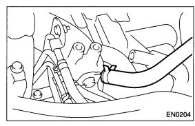
15) Disconnect the pressure hose from the intake duct.
