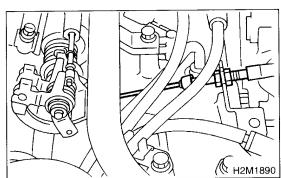
10) Remove the coolant filler tank. <Ref. to CO-51, REMOVAL, Coolant Filler Tank.>
