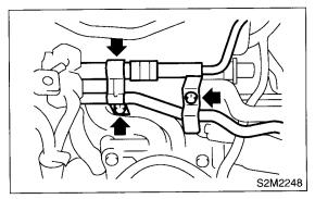
(4) Remove the bolts which secure the power steering pump bracket.
