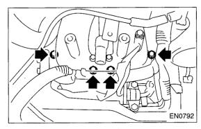
24) Remove the intake manifold.
